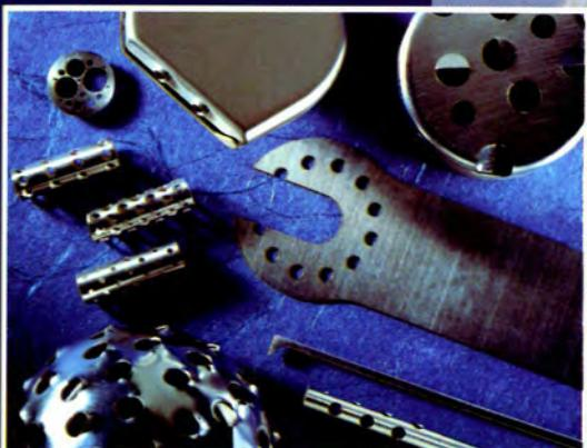
Laser cutting of difficult material such as hardened steel, ceramics and composite material can solve challenging manufacturing problems. Likewise, laser drilling of small controlled diameter holes in difficult materials has made it possible to design unique drug delivery systems and flow control orifices. Over a quarter billion precisely located 0.005" (0.13 mm) diameter holes have been produced for one particular application.
